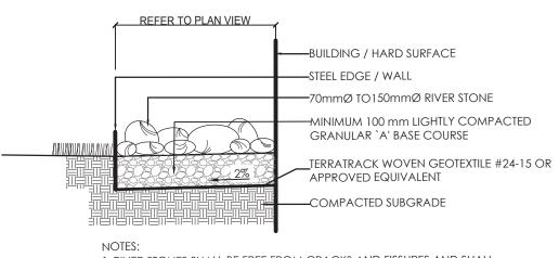
1. RIVER STONES SHALL BE FREE FROM CRACKS AND FISSURES AND SHALL BE FREE FROM SAND CLAY AND OTHER DELETERIOUS MATERIAL. 2. RIVER STONES SHALL BE LIGHTLY COMPACTED TO EMBED INTO
