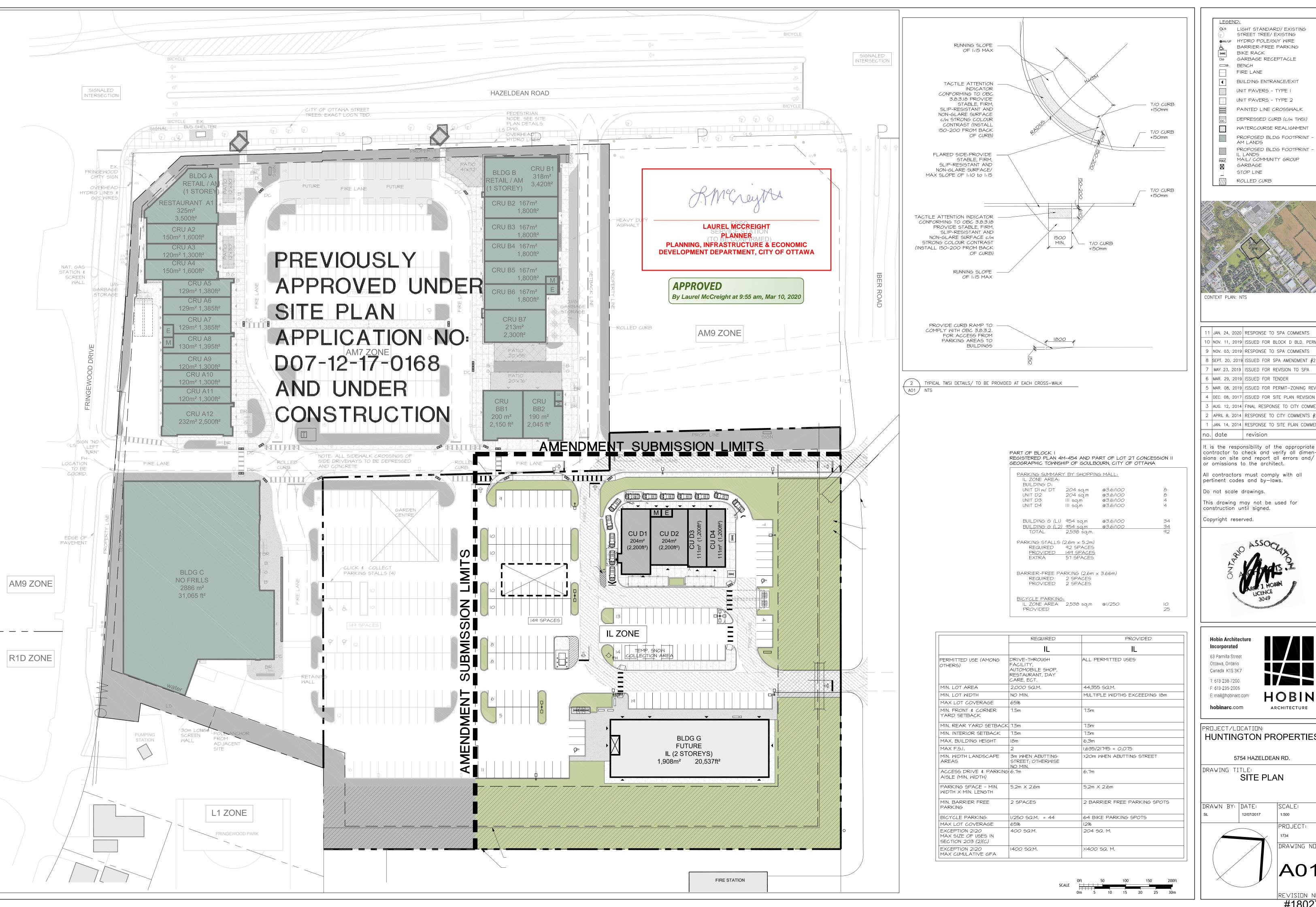
OLS LIGHT STANDARD/ EXISTING STREET TREE/ EXISTING •AN/UP HYDRO POLE/GUY WIRE BARRIER-FREE PARKING BIKE RACK GARBAGE RECEPTACLE BENCH FIRE LANE BUILDING ENTRANCE/EXIT UNIT PAVERS - TYPE I UNIT PAVERS - TYPE 2 PAINTED LINE CROSSWALK DEPRESSED CURB (c/w TWSI) WATERCOURSE REALIGNMENT PROPOSED BLDG FOOTPRINT PROPOSED BLDG FOOTPRINT -MAIL/ COMMUNITY GROUP GARBAGE STOP LINE ROLLED CURB
