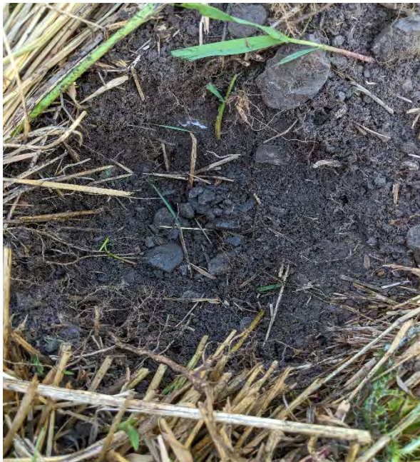
Image 10: View of disturbed test pit, showing sand fill with gravel inclusions (CY 2019).
