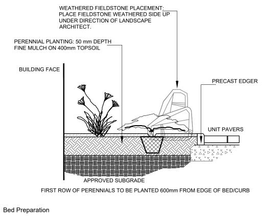
.1 EXCAVATE OR PLACE FILL FOR PLANTING BED TO PROVIDE 400mm MINIMUM DEPTH OF PLANTING MEDIUM. .2 PLACE 150mm PLANTING MEDIUM ON APPROVED SUBGRADE AND CULTIVATE INTO TOP 150mm OF APPROVED SUBSOIL. APPROVED SUBJOL.
