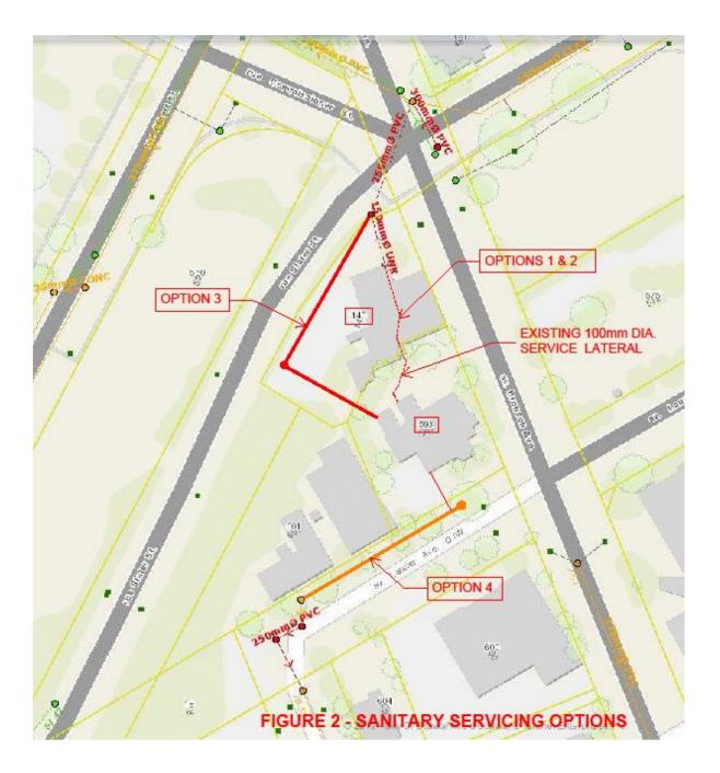
The Option 3 was chosen through discussions with the City of Ottawa. Therefore, the proposed residential development will be serviced by a new 200mm dia. sanitary sewer that will be routed through the 140 Bronson property and connected to the existing 250mm dia. sanitary sewer at the corner of Slater Street and Bronson Avenue.
