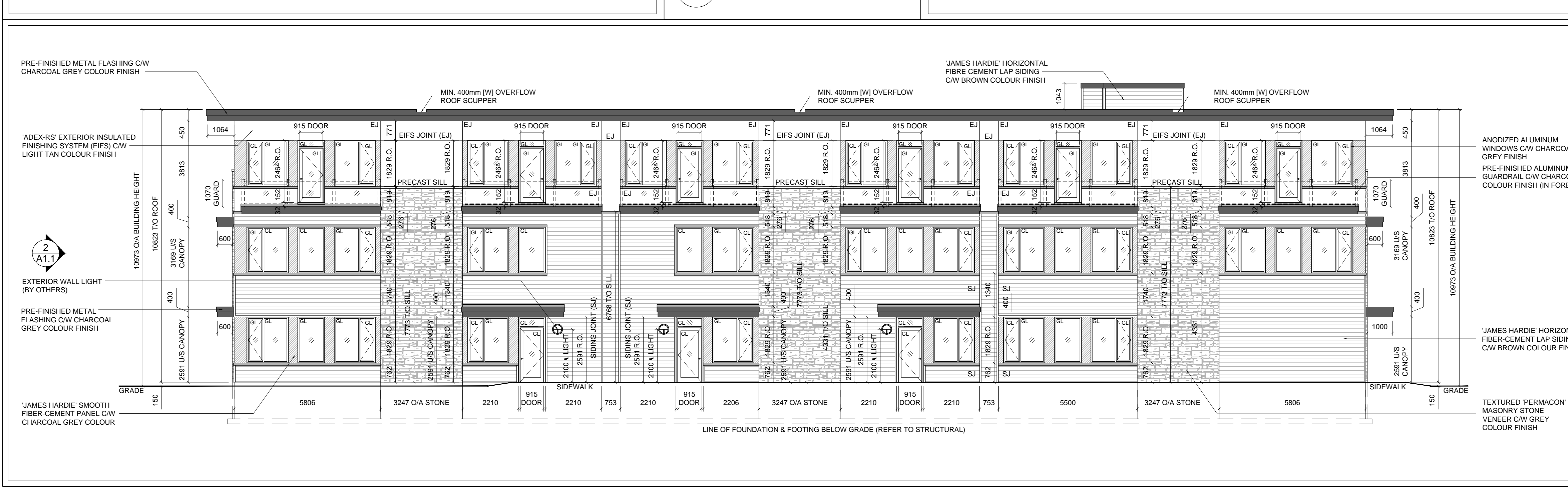
2 North Elevation A1.1 1:100
