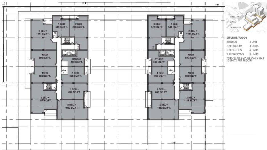
FIGURE 31: PROPOSED FLOOR PLAN - WEST SIDE - LEVEL 7-9 | EAST SIDE LEVEL 7 - 15 - PHASE 2
