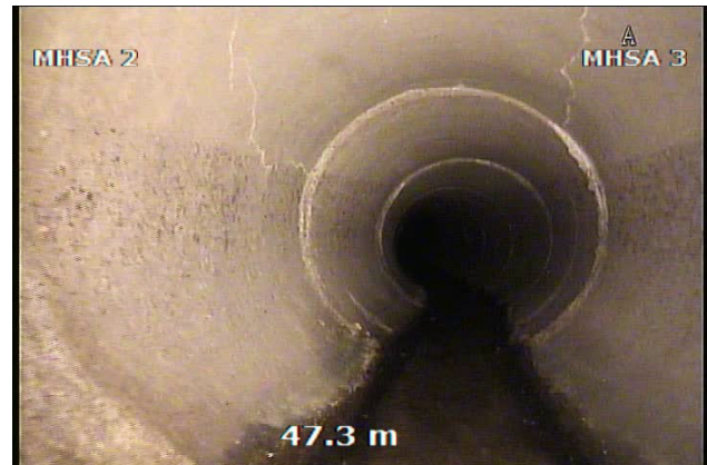
Figure 15 – Minor cracking at 9 and 1 o'clock
