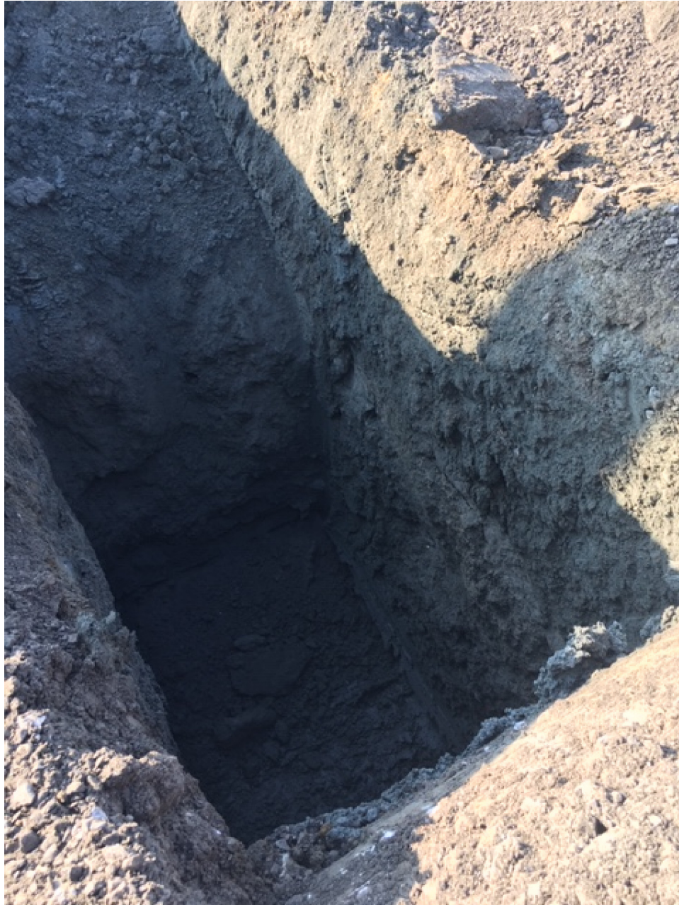
TP-2 - Silty clay fill is relatively compact and similar to native soil. Native silty clay deposit encountered at approximately 3.2 m depth.
