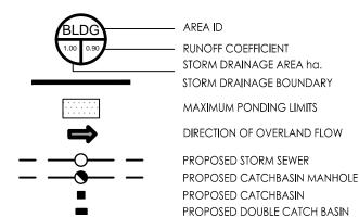
PROPOSED PERFORATED SUBDRAIN \_\_\_\_\_ EXISTING STORM SEWER \_ \_ \_ \_ \_ EXISTING CATCHBASIN MANHOLE EXISTING CATCHBASIN EXISTING SUBDRAIN CATCHBASIN FUTURE STORM SEWER FUTURE CATCHBASIN MANHOLI
