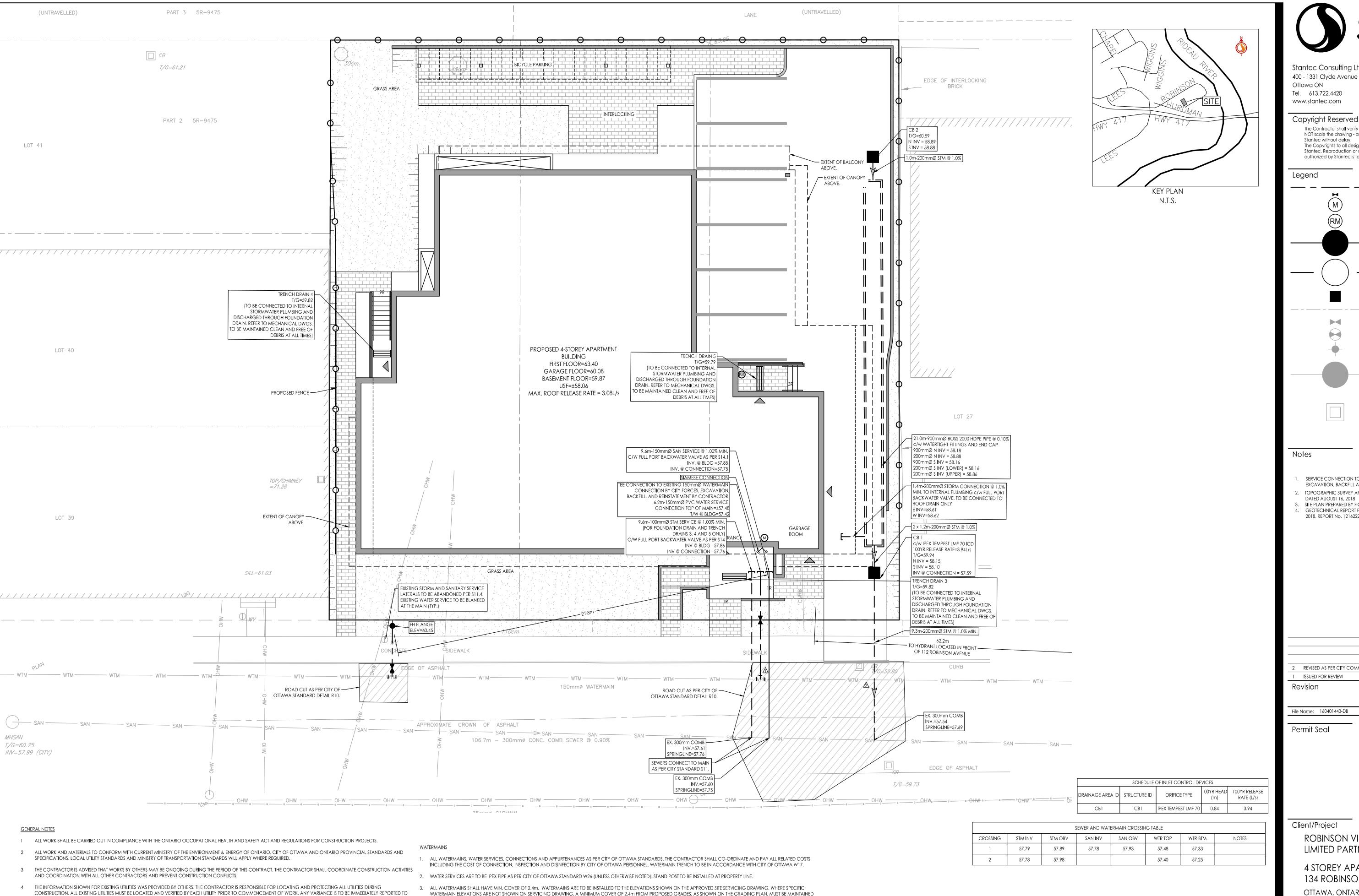
WATERMAIN ELEVATIONS ARE NOT SHOWN ON SERVICING DRAWING, A MINIMUM COVER OF 2.4m FROM PROPOSED GRADES, AS SHOWN ON THE GRADING PLAN, MUST BE MAINTAINED AT ALL TIMES. IN PREGRADE AREAS COVER TO BE FROM PREGRADED ELEVATIONS.
