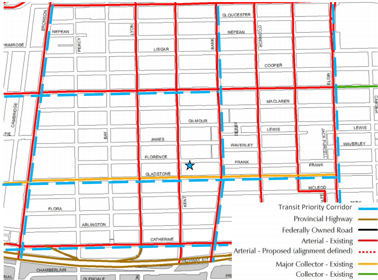
Figure 3. Urban Road Network, Markup of Schedule F of the City of Ottawa Official Plan
