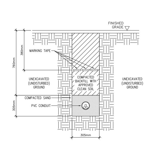
B ELECTRICAL UNDERGROUND DETAIL - UNDER LANSCAPING/LAWN SCALE:NOT TO SCALE
