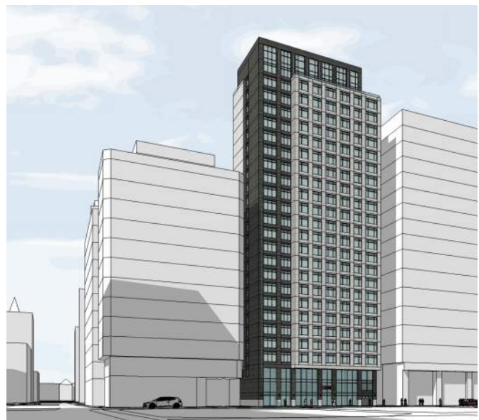
Figure 1.26 Volume projection used to frame the base and roof of the building
