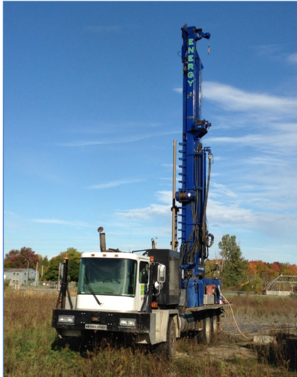
Air Rock Drilling rig at 6045 Bank Street
