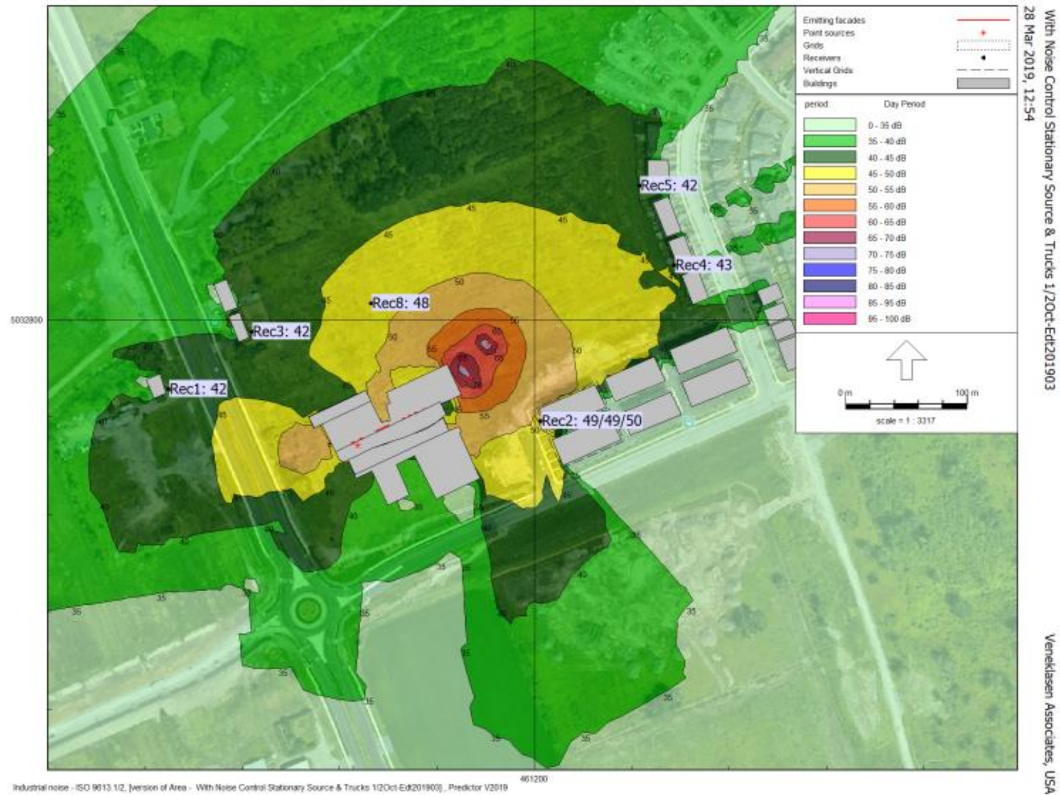
Figure 8 – Noise Contours with Noise Control Employed Day/Evening time (Stationary Sources)
