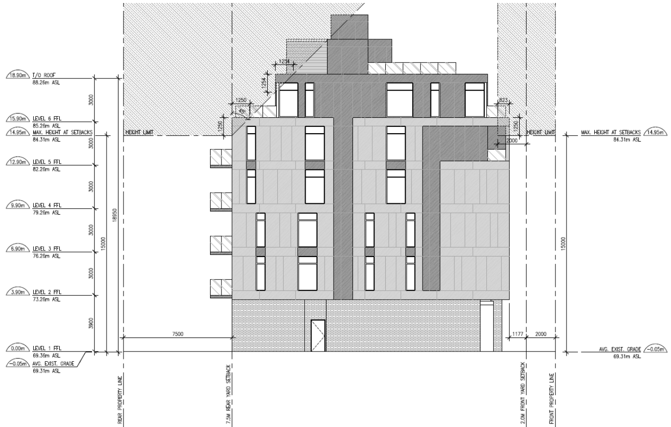
Figure 11: Elevation drawing showing required upper-storey stepbacks
