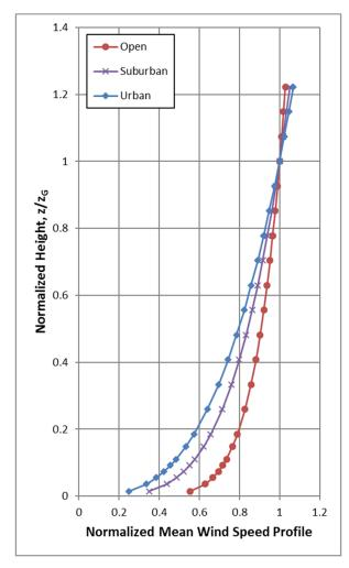
**Figure A1: Mean Wind Speed Profiles**
