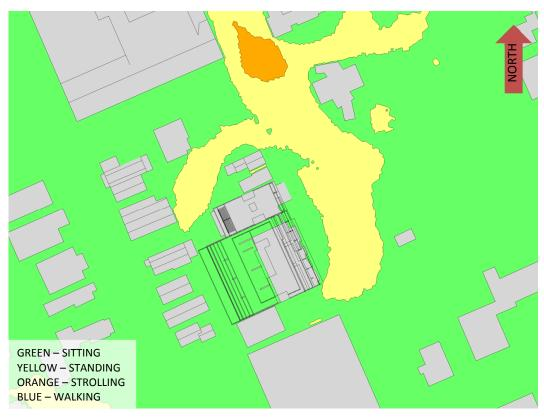
FIGURE 3A: SPRING - GRADE-LEVEL PEDESTRIAN WIND CONDITIONS
