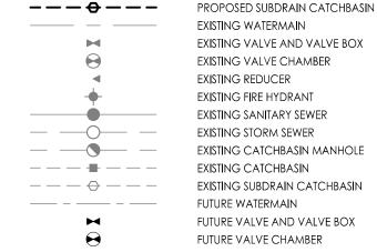
EXISTING STORM SEWER EXISTING CATCHBASIN MANHOLE EXISTING CATCHBASIN EXISTING SUBDRAIN CATCHBASIN FUTURE WATERMAIN FUTURE VALVE AND VALVE BOX FUTURE VALVE CHAMBER FUTURE REDUCER FUTURE FIRE HYDRANT
