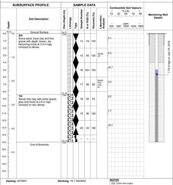
Site Datum: Top of casing of drilled test well on site (100.00 m).
