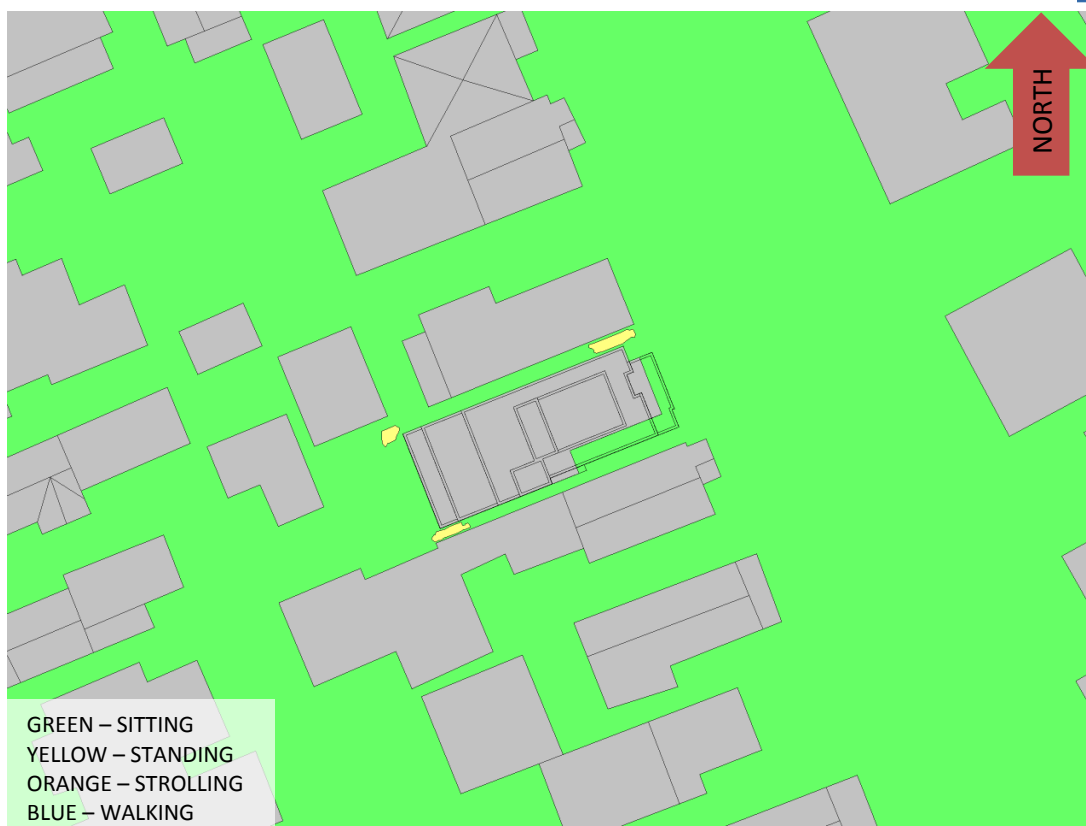
FIGURE 3A: SPRING – GRADE-LEVEL PEDESTRIAN WIND CONDITIONS
