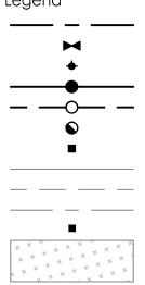
PROPOSED WATERMAIN PROPOSED VALVE BOX PROPOSED FIRE HYDRANT PROPOSED SANITARY SEWER PROPOSED STORM SEWER PROPOSED CATCHBASIN MANHOLE PROPOSED CATCHBASIN EXISTING SANITARY SEWER EXISTING STORM SEWER EXISTING WATERMAIN EXISTING CATCHBASIN EXISTING ASPHALT LIMITS
