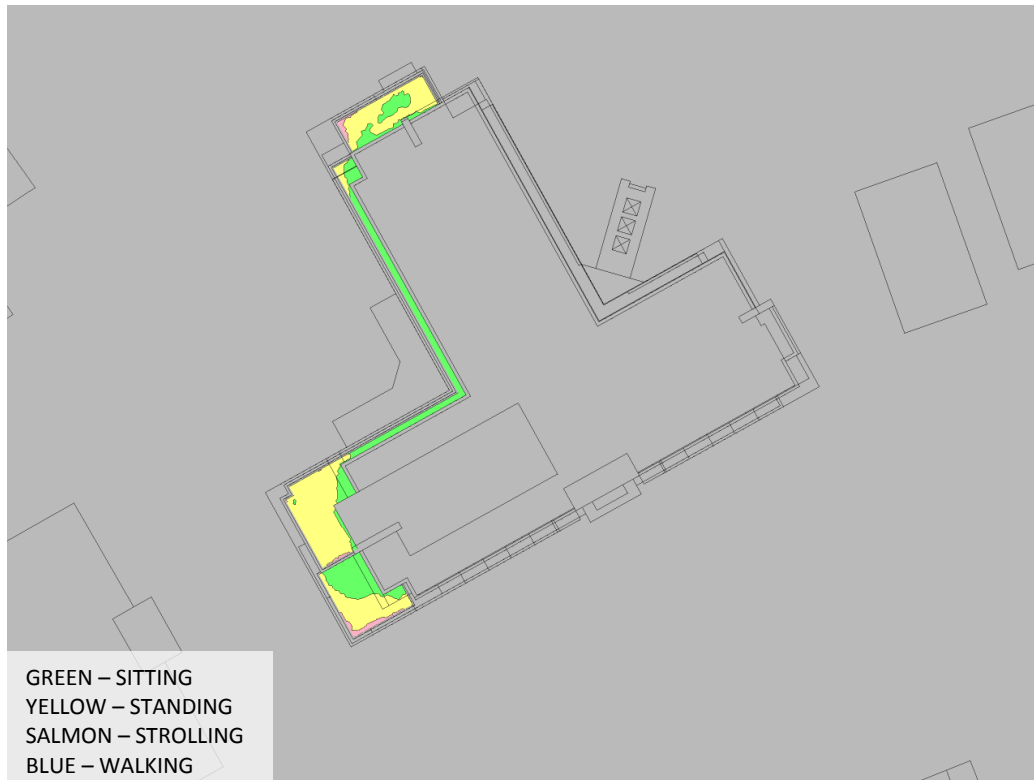
FIGURE 3B: SPRING – OUTDOOR AMENITY AREA WIND CONDITIONS
