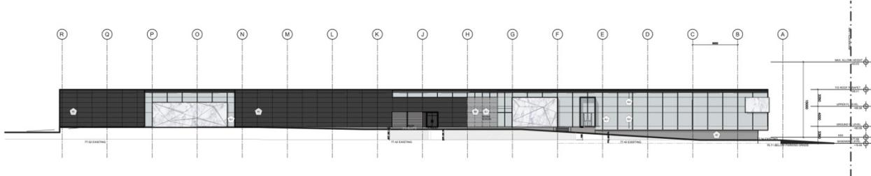
A simple material palette of 3 elements has been proposed. It includes dark precast panels, curtain wall, as well as natural marble panel. The dark precast concrete panels are a counterpart to the full height glass and punctuations of elegant stone elements. These stone elements continue from the exterior façade into the showroom area.
