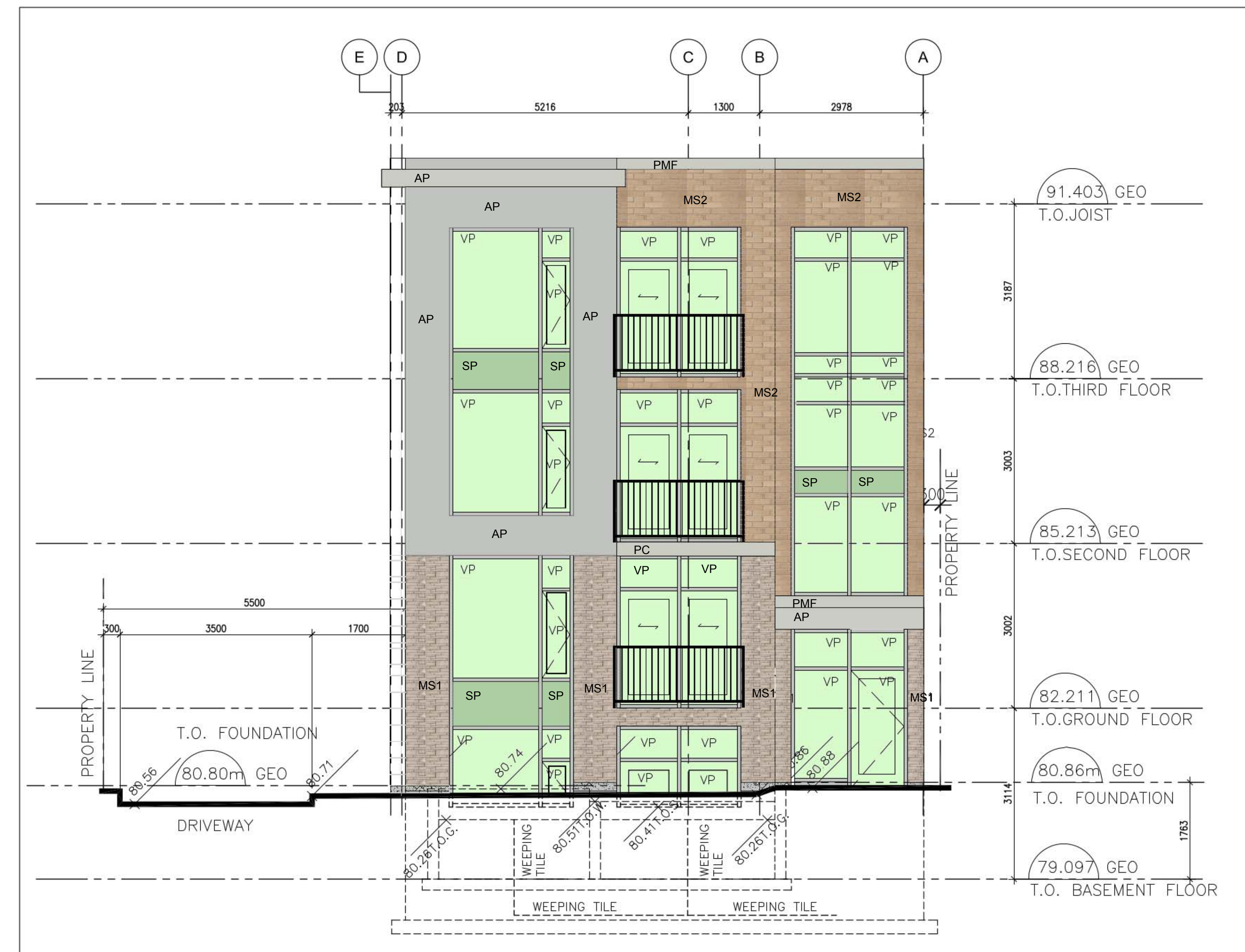
1 EAST ELEVATION (REAR) A302 SCALE: 1:50
