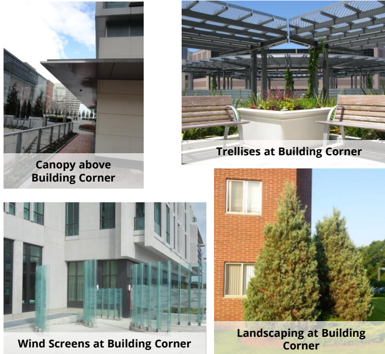
Image 8 – Examples of Wind Control Features at the Parking Lot and at the Northwest Building Corner
