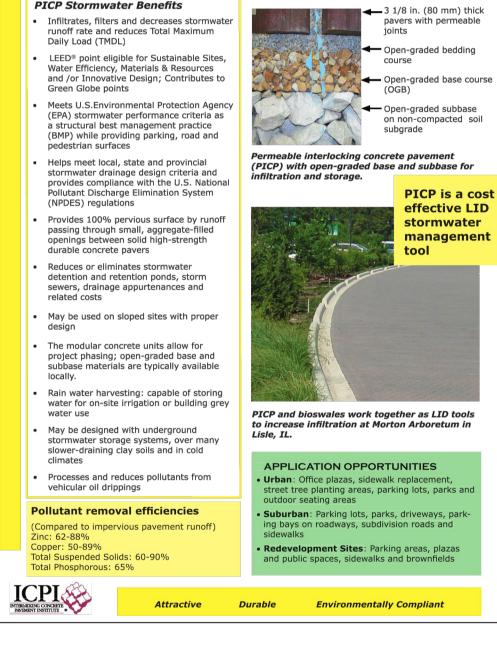
PERMEABLE INTERLOCKING CONCRETE PAVEMENT (PICP)
