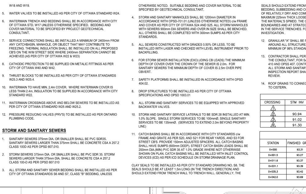
SEALS SHOULD EXTEND FROM THE FROST LINE AND FULLY PENETRATE THE BEDDING SUBBEDDING AND COVER MATERIAL. THE BARRIERS SHOULD CONSIST OF RELATIVELY DRY AND COMPACTABLE BROWN SILTY CLAY PLACED IN MAXIMUM 225mm THICK LOOSE LAYERS COMPACTED TO A MINIMUM OF 95% OF THE MATERIAL'S SPMDD. THE CLAY SEALS SHOULD BE PLACED AT THE SITE BOUNDARIES AND AT STRATEGIC LOCATIONS AT NO MORE THAN 60m INTERVALS IN THE SERVICE TRENCHES. FOR DETAILS REFER TO GEOTECHNICAL
