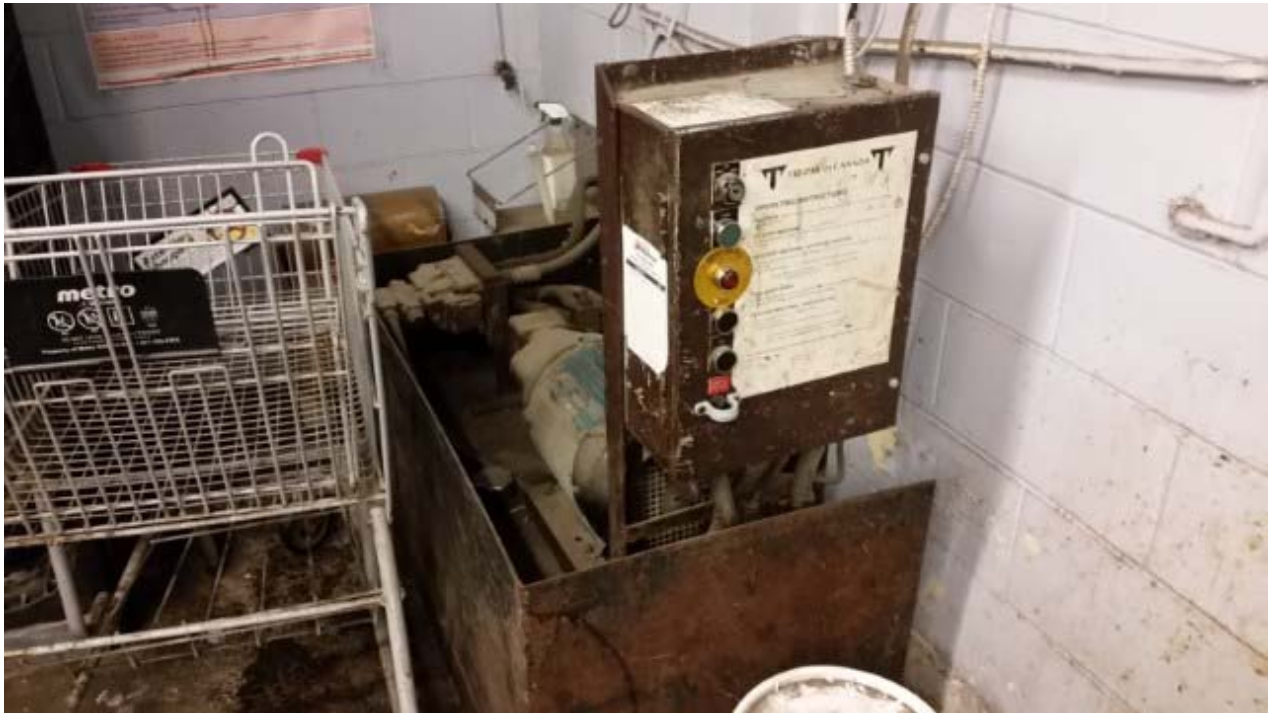
Photo 15: Metro's hydraulic garbage compactor unit.
