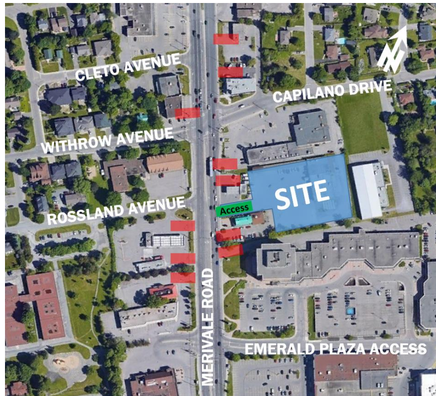
Figure 3: Adjacent Driveways within 200m of Site Access
