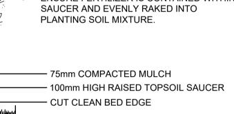
— SOD AS SPECIFIED - PLANTING SOIL MIXTURE AS SPECIFIED. TAMP SOIL MIXTURE IN LAYERS TO PREVENT AIR POCKETS - CUT AND REMOVE ALL WIRE, BURLAP, ROPE AND TWINE FROM TOP  $\frac{1}{3}$  OF ROOT BALL
