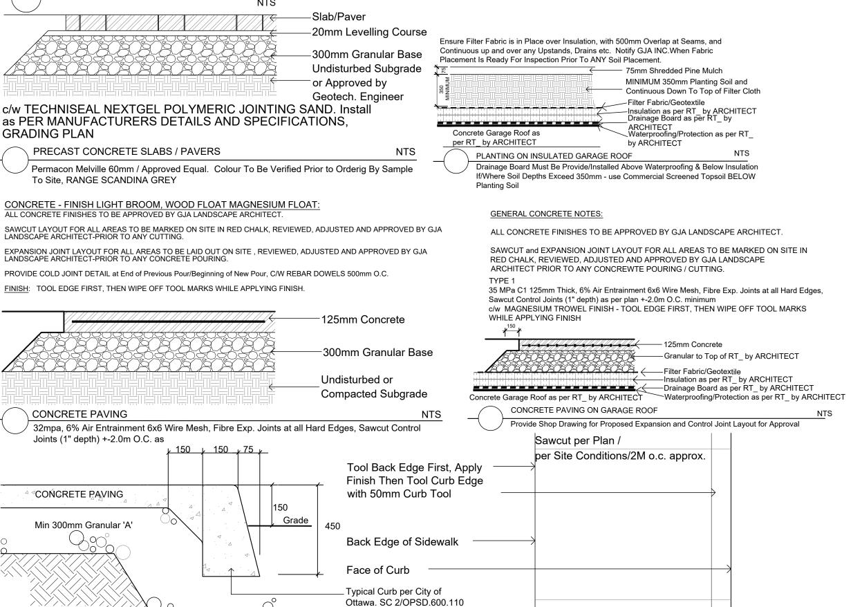
NO Dummy Joints/Visible Tooled Edges Except for Curb Edge
