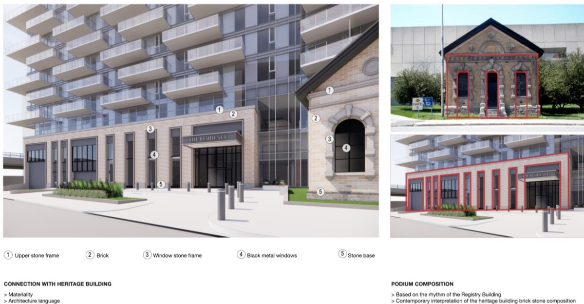
Figure 19: Illustrates the relationship between the proposed development and the CRO. Given the differences in scale, it is considered key to the visual compatibility of the overall development that the materiality, and colour of the base of the high-rise act as a backdrop to the CRO without overwhelming it. Introducing the salmon yellow
