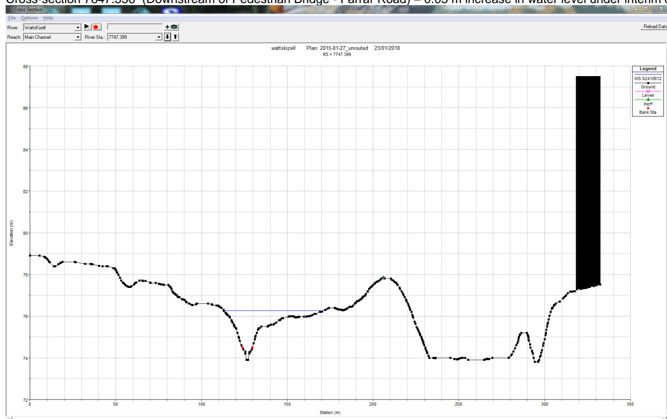
Cross-section 7747.399 (Downstream of Pedestrian Bridge - Farrar Road) – 0.05 m increase in water level under interim conditions (right side)
