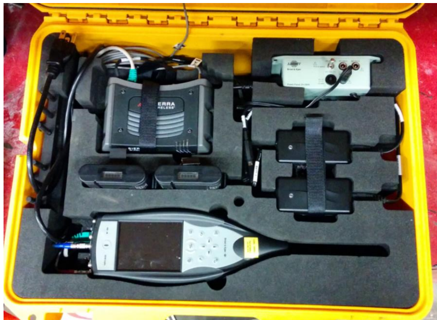
PHOTOGRAPH 3: NOISE MONITOR STATION
