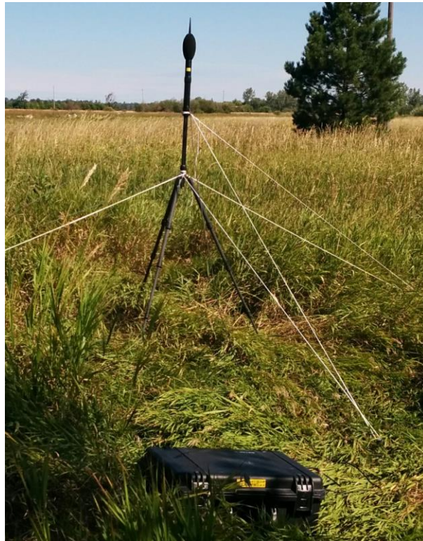
PHOTOGRAPH 1: NOISE MONITOR STATION
