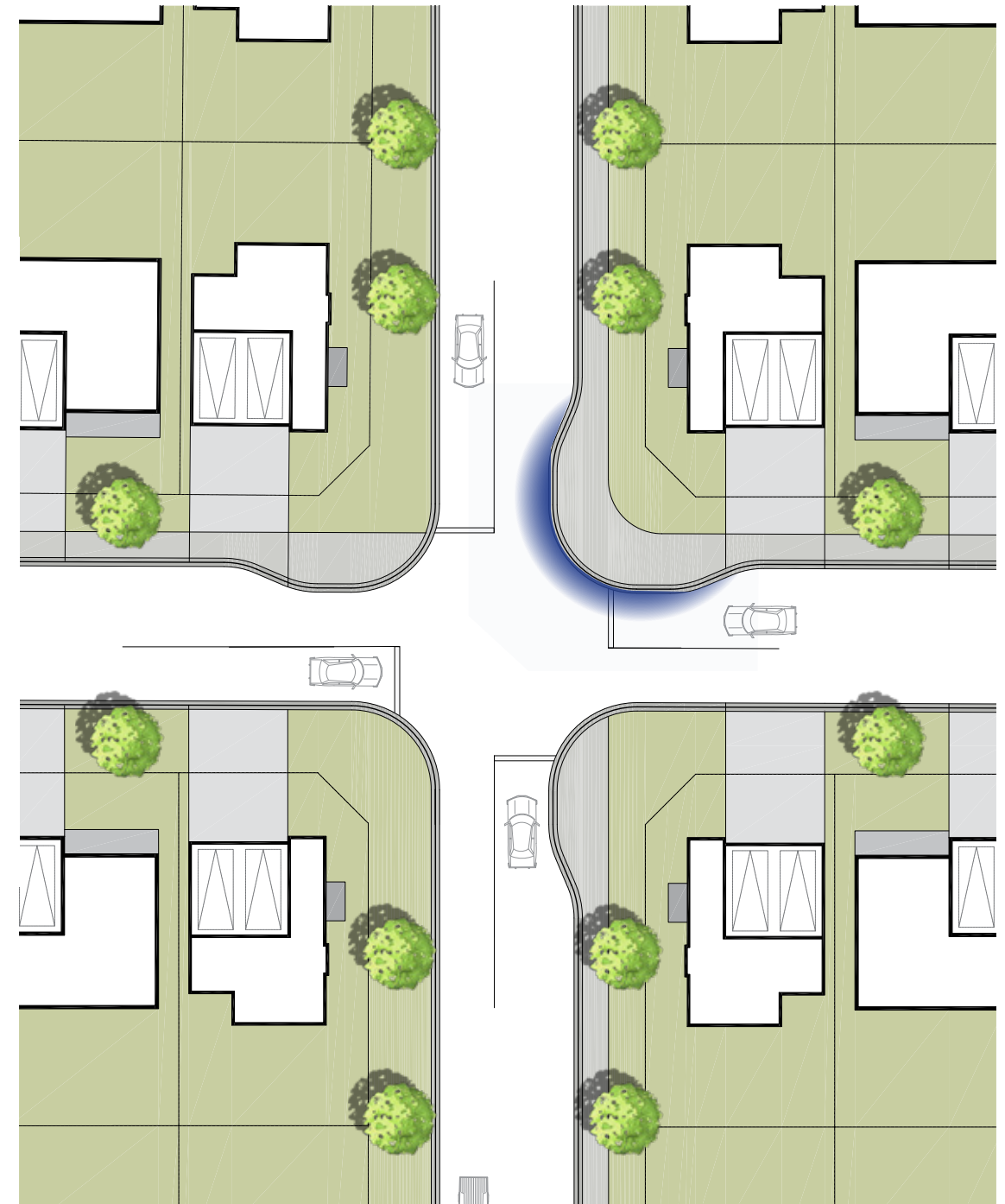
Figure 31 Double Bulb-Out at Intersection
