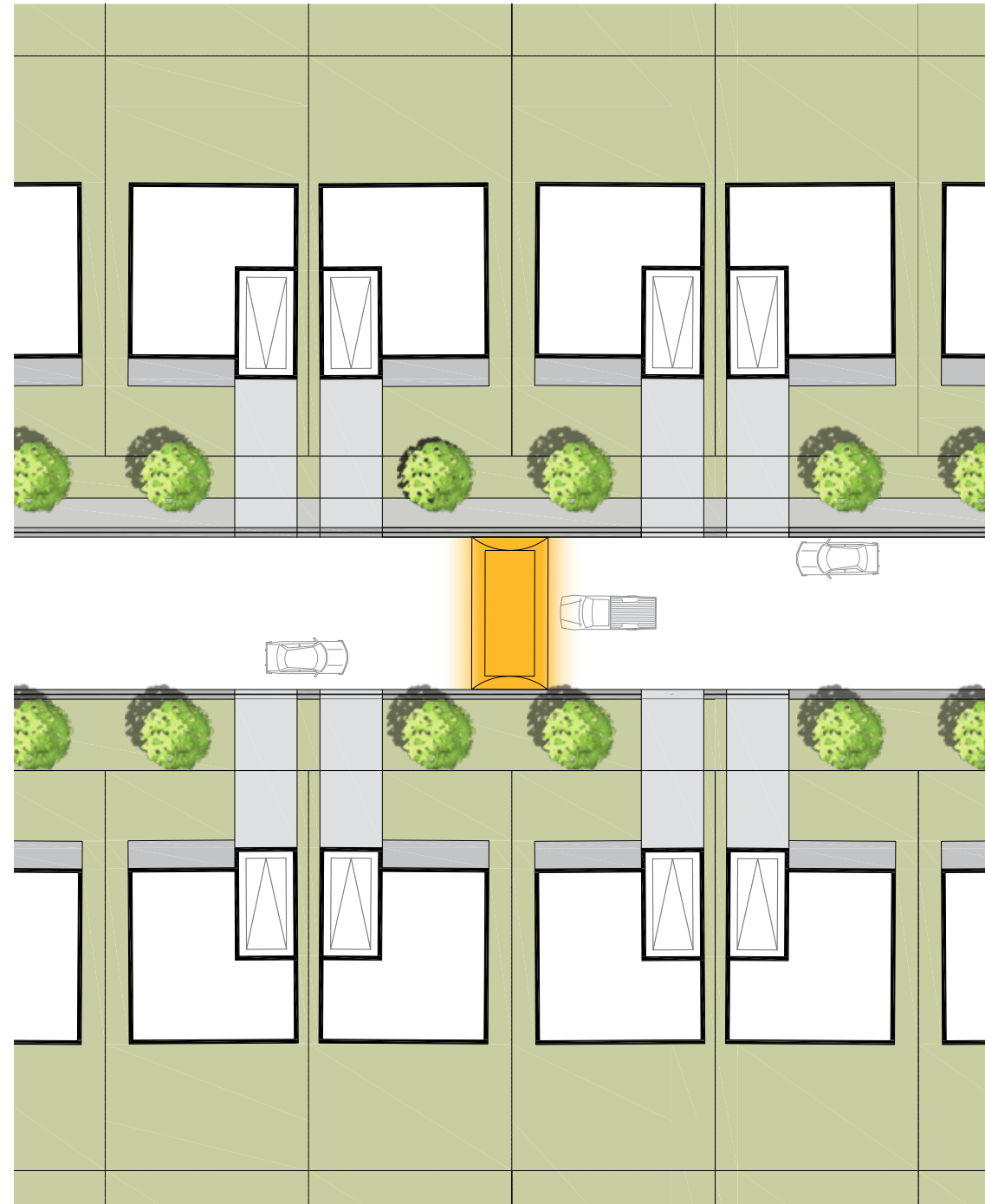
Figure 32 Speed Hump on Local Street
