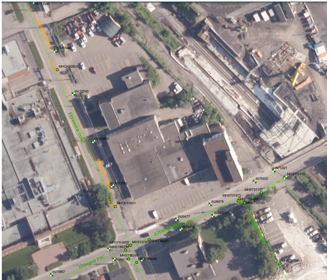
Figure 4-1 Existing Storm Sewer Services
