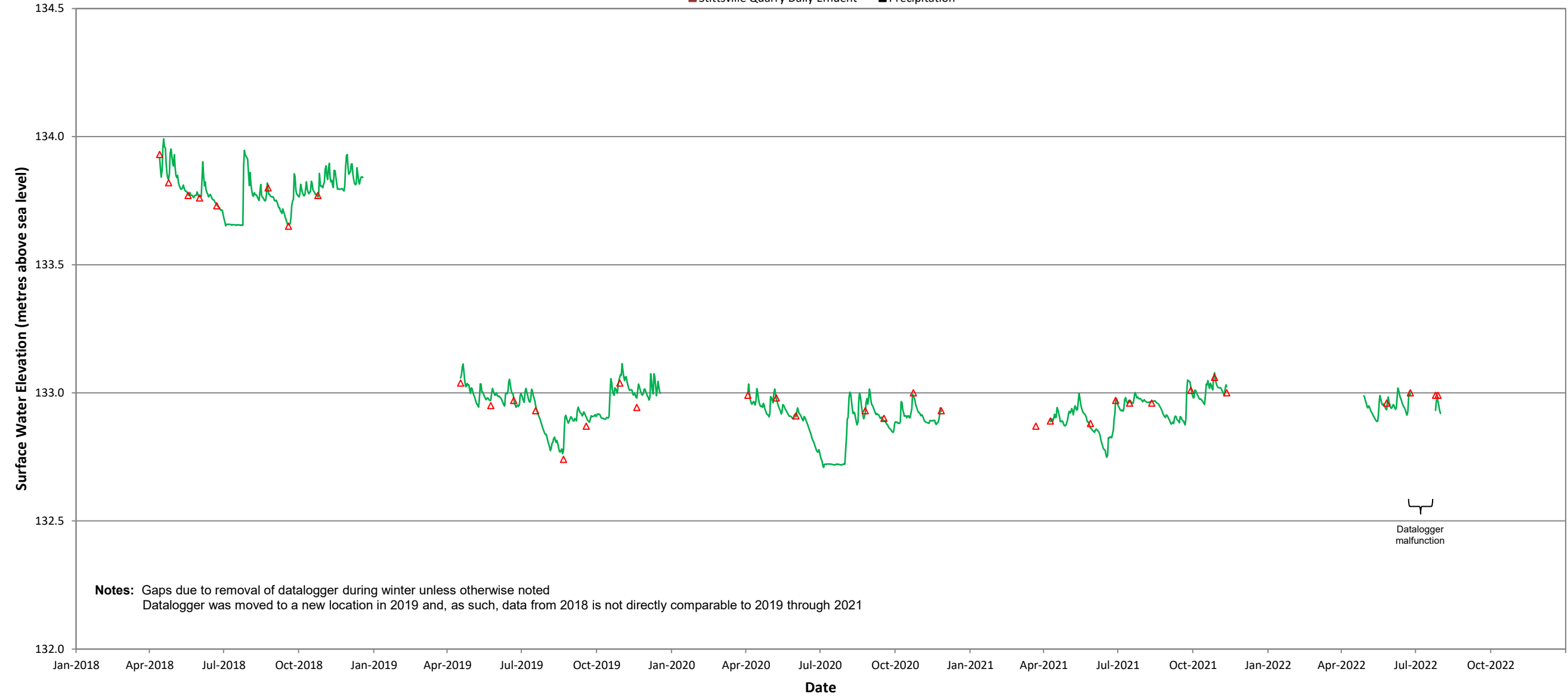
— SG-4 Daily Average Water Elevation (Datalogger) ▲ SG-4 Surface Water Elevation (Staff Gauge)
