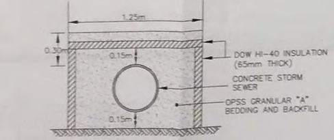
**STORM SEWER INSULATION DETAIL**
