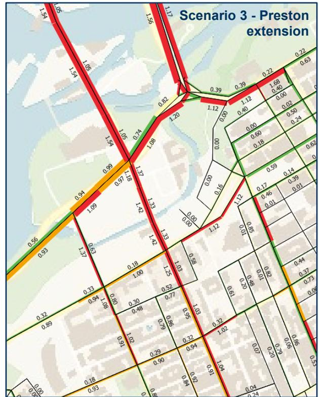
Figure 23: PM Peak Hour EMME Model v/c Ratio
