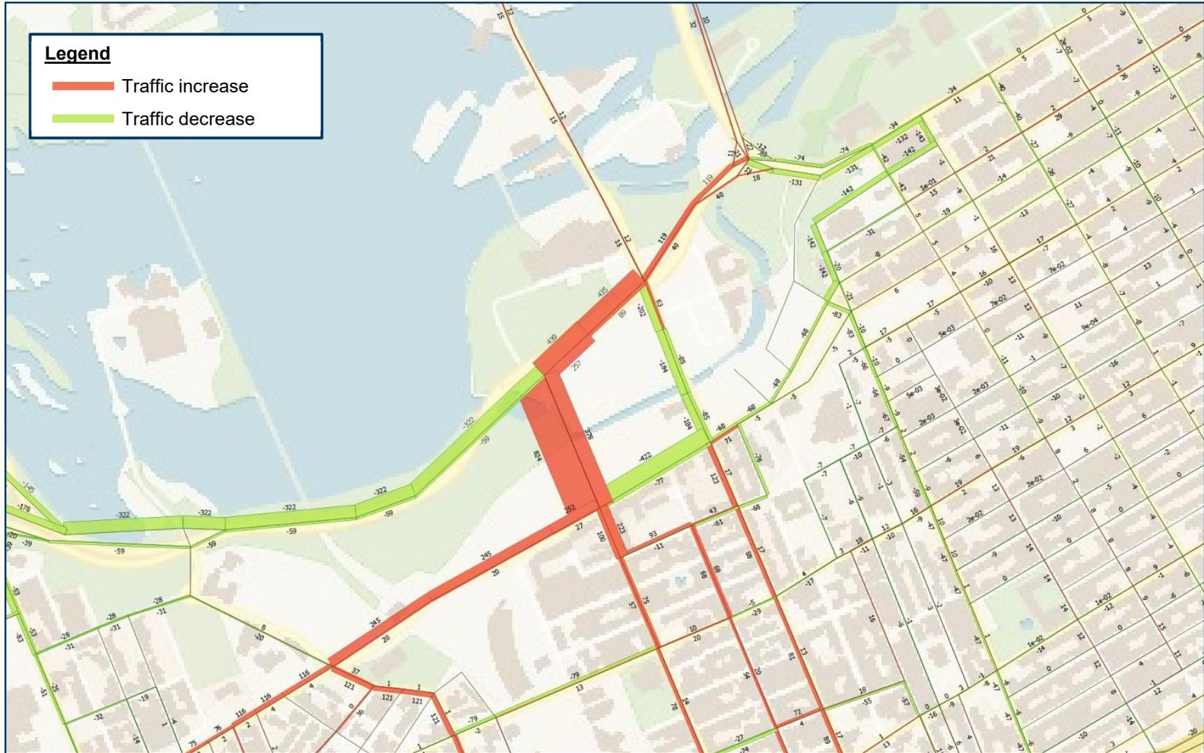
Figure 25: Preston Extension Traffic Diversion – Road Network, AM Peak Hour
