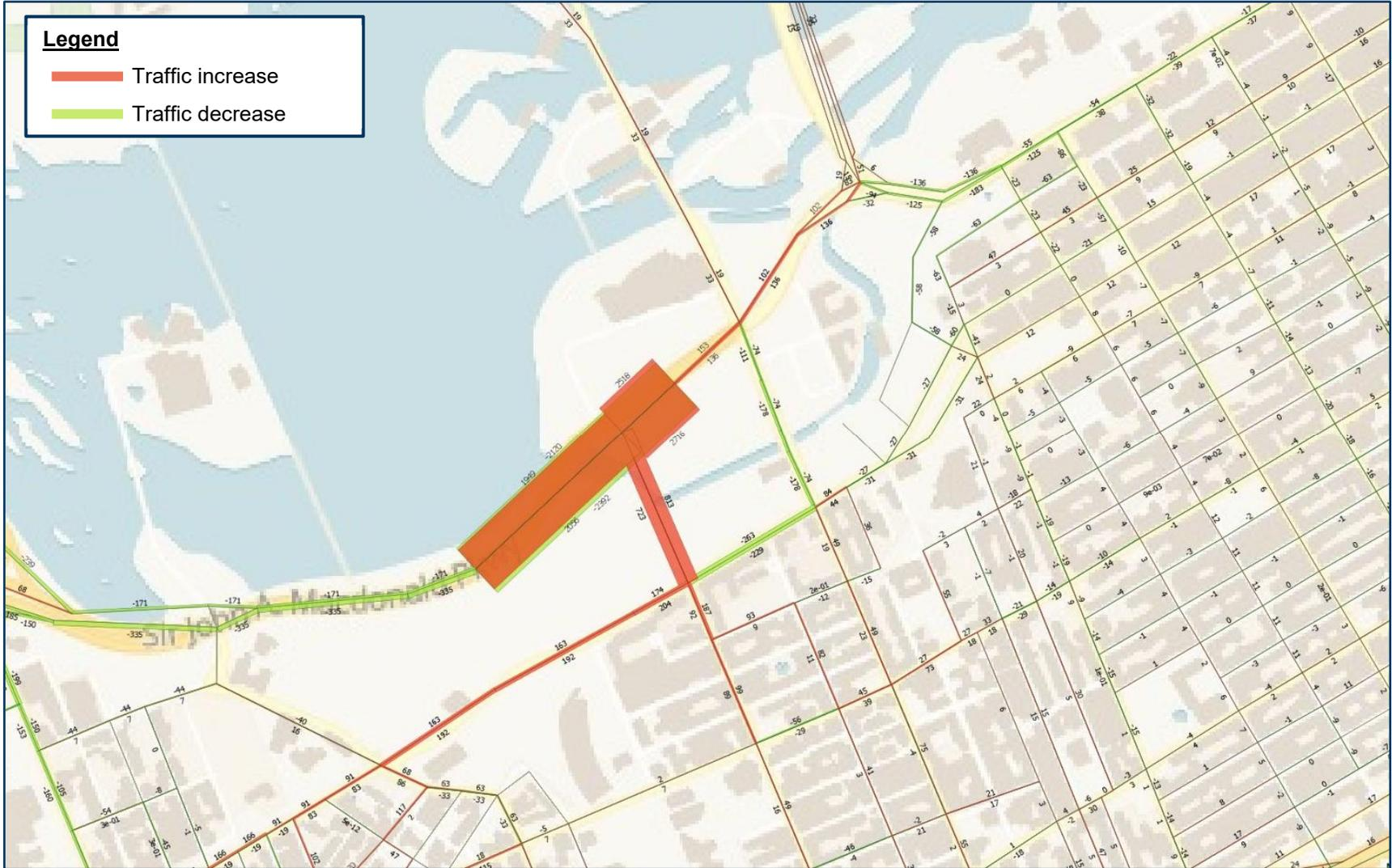
Figure 27: Preston Extension Traffic Diversion – Road Network, PM Peak Hour
