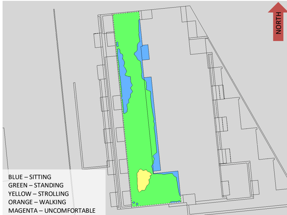
FIGURE 4A: SPRING – WIND COMFORT, LEVEL 17 AMENITY TERRACE
