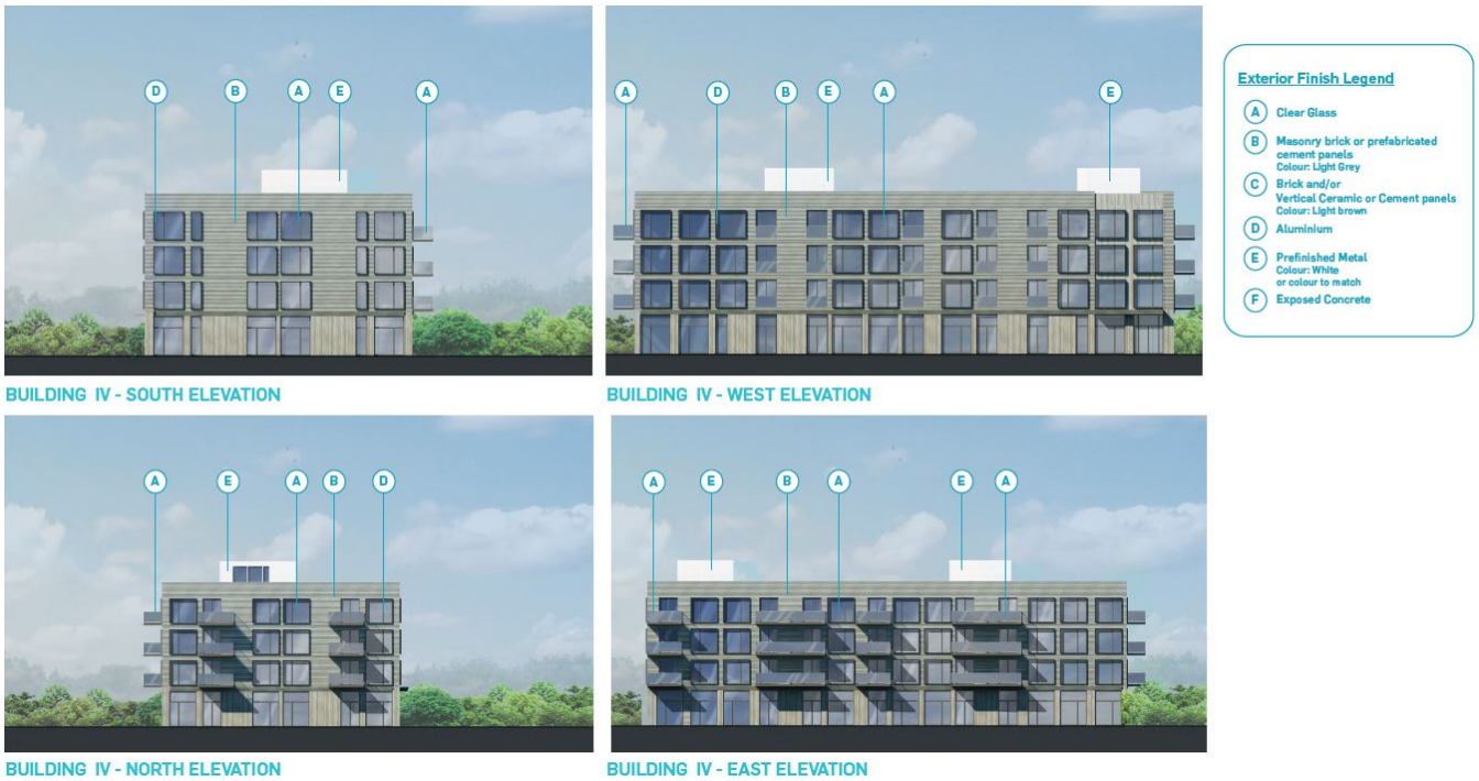
Figure 33. Building IV design details.
