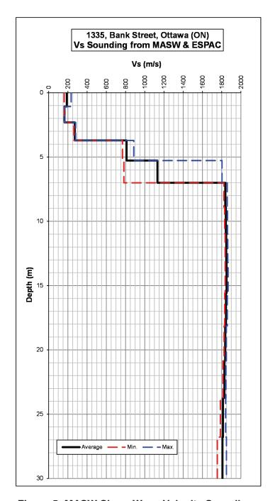
Figure 5: MASW Shear-Wave Velocity Soundings
