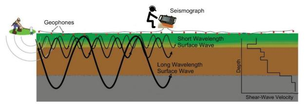
**Figure 3: MASW Operating Principle**
