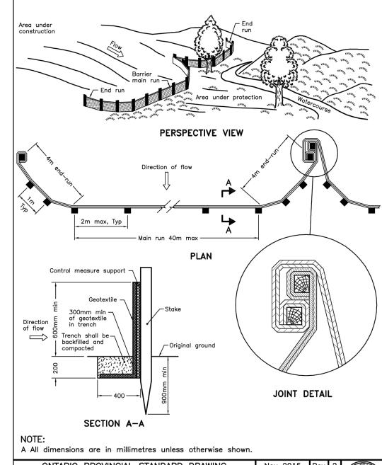
Nov 2015 Rev 2 STAN ONTARIO PROVINCIAL STANDARD DRAWING HEAVY-DUTY SILT FENCE BARRIER OPSD 219.130
