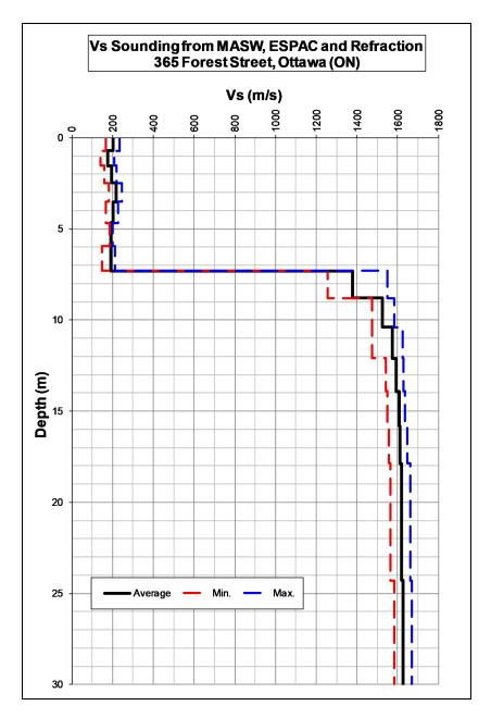
Figure 5: MASW Shear-Wave Velocities Sounding
