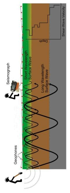
Figure 3: MASW Operating Principle
