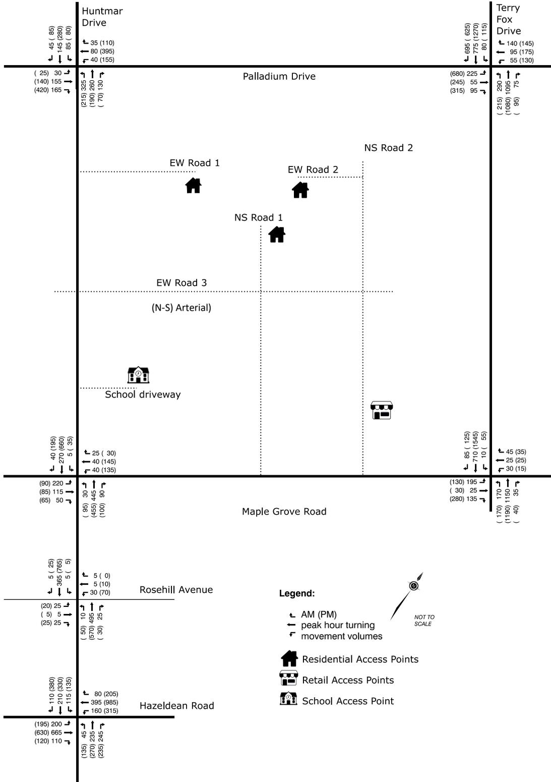
Figure 11: Existing Lane Geometry and Traffic Control
