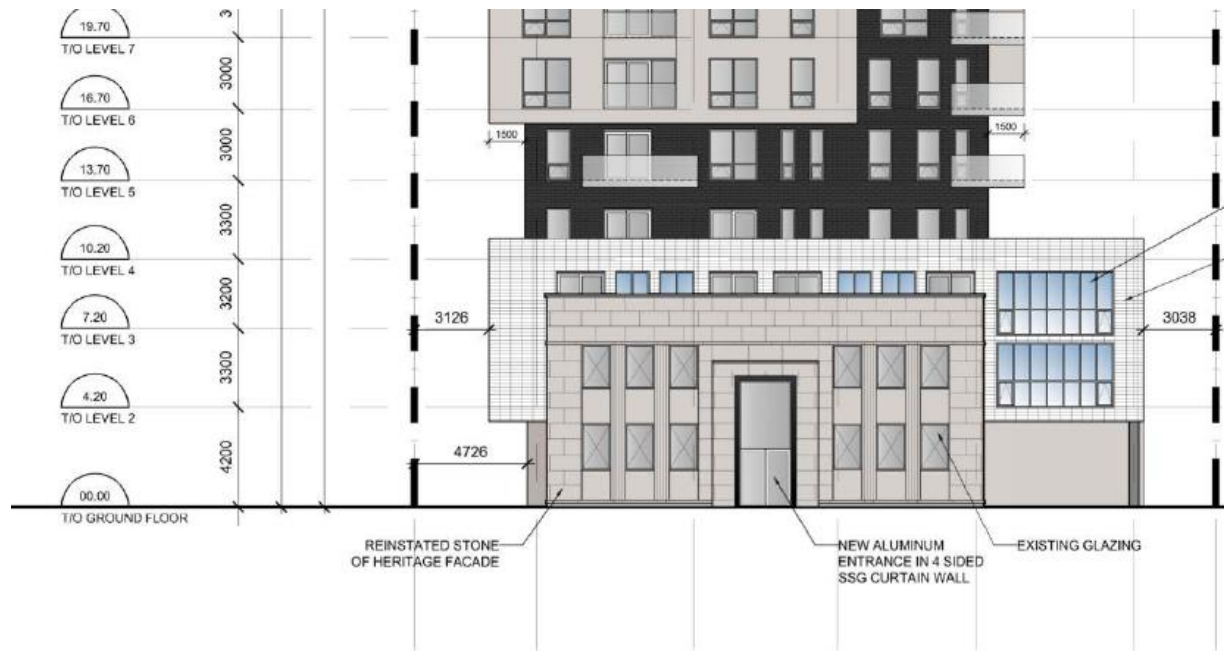
Figure 21: View of the south façade illustrating the relationship of the original façade as part of the podium distinct from the main tower. The tower will step back approximately 5.0m from the front façade of the entrance foyer as part of a distinct podium. The east side of the development site has a 3.66m right of way and the west side has a 1.63m right of way.
