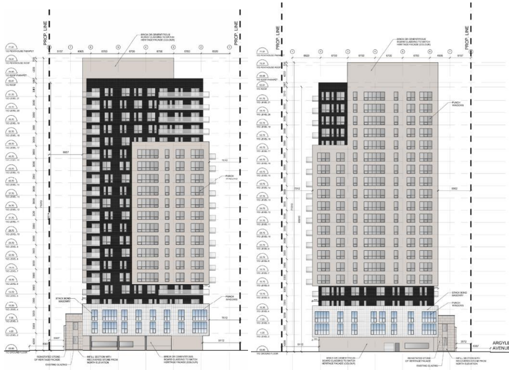
Figure 25 and 26: Rendered elevations of the proposed tower looking both west and east are well articulated. The use of tan brick or cementitious board in a colour matching the limestone façade helps to anchor the building and connect it to the upper levels of the tower. The original building is set proud of the main tower and retains its position to the street.
